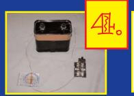
Set up the experiment with a switch (as shown), or connect one lead from the galvanometer to a battery terminal. Create your own switch by touching the other lead from the galvanometer to the opposite battery terminal when the current needs to be turned on. Remember: most "bare" copper wire has a insulating covering of varnish or paint. Be sure to sand the ends of each section of wire to ensure that good electrical connections are made.
